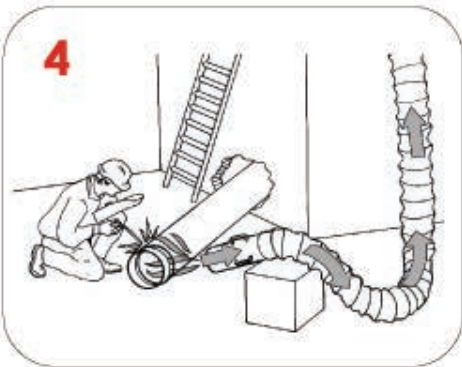
4 Suction of welding fumes in indoor works
