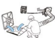
Aspiration in manholes and closed ambients
