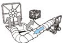
Ventilation of manholes and closed ambients
