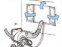
The fans can be positioned directly in the closed environment
